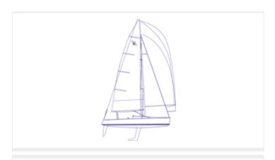
Recognized **ISAF Status** 525 kg max ####change Year of status Keelboat Type 525 kg max No. of Crew Bruce Farr Designer GRP **Hull Material** 0 **Number of Trapeze** 9.43 m **Hull Length** 2.1 m **Beam Length** 35.2 m2 Mainsail Area 17.7 m2 **Headsail Area** 91 m2 Spinnaker Area 1948 kg **Boat Weight** 938 kg **Ballast Weight**
